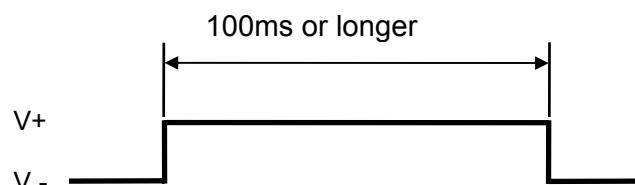
In most cases the Brake Signal can be omitted. The example program shows how a Brake Signal can be implemented under MS-DOS. The example program consists of two procedures where the inner procedure "LCR\_Brake" is called by the outer procedure ("STX\_ComReset"). Note that this program will directly address the comport chip. There may be operating systems that will not allow the chip to be addressed directly.
