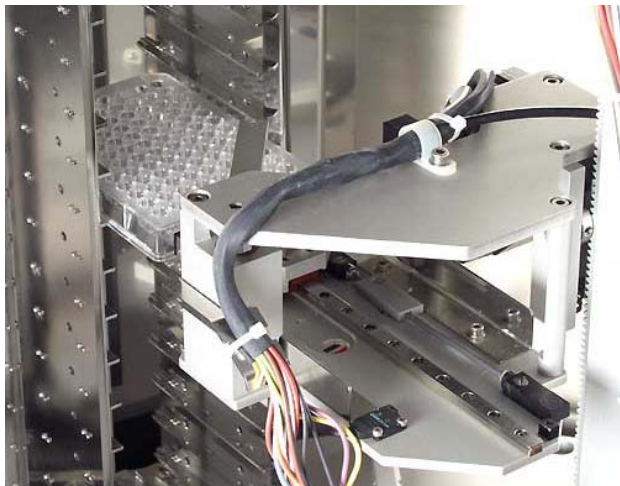
Figure 4-1 Plate transfer Stack - Lift
