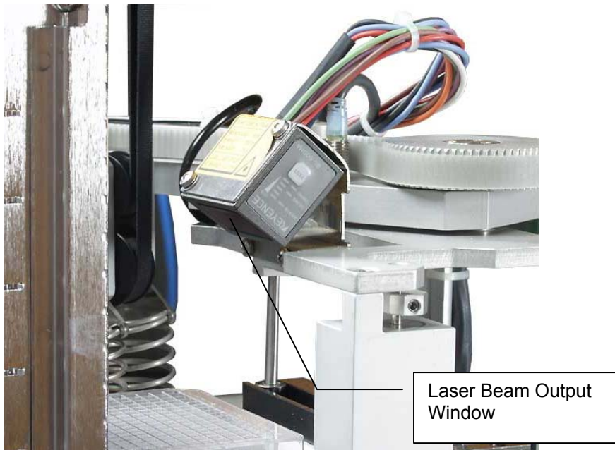
Figure 5-1 Position of Laser Beam Output Window
