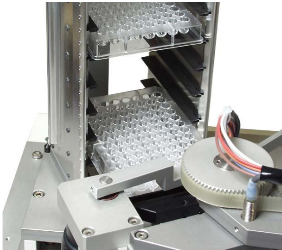
Figure 4-1 Plate transfer Stack - Lift
