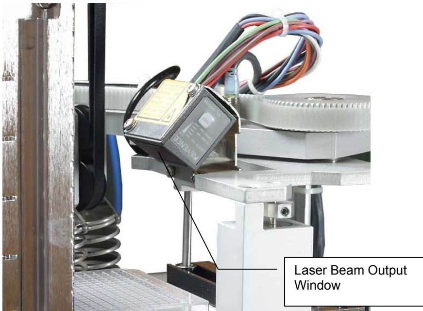
Figure 5-1 Position of Laser Beam Output Window
