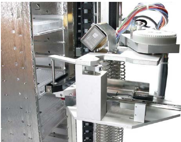
Figure 4-1 Plate transfer Stack - Lift
