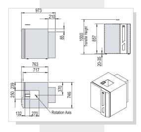
The periscope delivery shovel presents the plate to the top of the work surface. With work space at a premium, the STR will save valuable space for other components above your system and gives you a more aesthetically pleasing compact appearance.
