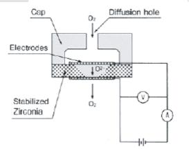
By attaching a cap with an aperture on one side (cathode) of the disc, the gas diffusion is limited and the saturated current is observed. It is tamed "limiting current". The limiting current is proportional to the ambient oxyen concentration.
