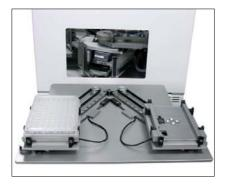
The parallel slide station design allows a LiCONiC Unit to be integrated with an external liquid handler without the need of an additional robot. With its precise stopping point it ensures that the devices need to be taught only once for accurate load and retrieval of the storage plates. The transfer nest is spring loaded to ensure the longevity of the liquid handling tips.
