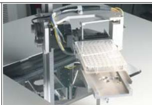
The LPR240 will hold up to 242 MTP with 23 mm pitch. It is ideal for multiple cassette/sample configurations. With its top loading functionality the unit sits entirely under the workstation or liquid handler deck. Multiple transfer-station can be used to increase production and throughput.
