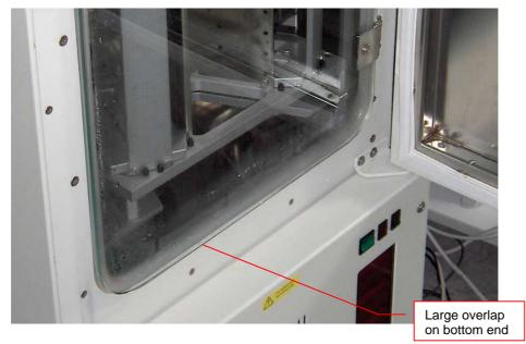
You may easily correct this by loosen the attachment screws of the hinges, lift-up the door up and re-tighten the screws again.
