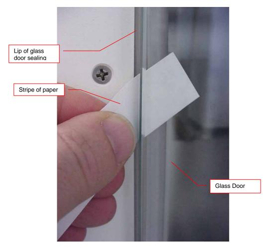
There should be slight resistance when moving paper along the seal. In case of a gap there is no more friction. It is sometimes helpful open the glass door before moving the paper to another location.
