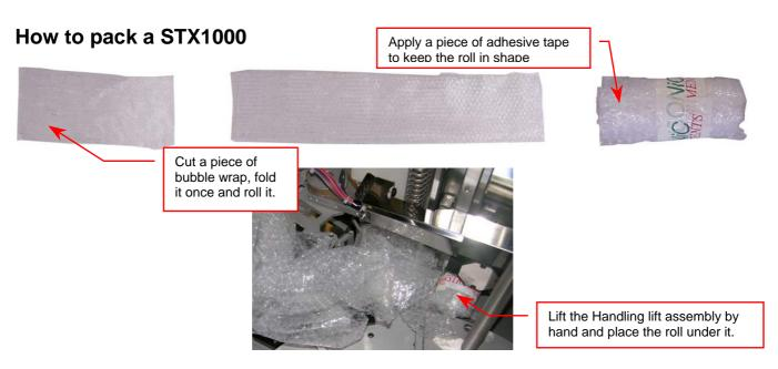
Secure the Handler with air pad foil and safe the carrousel with the transport lock and etafon pads.
