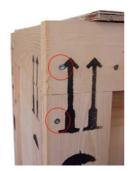
Next step, screw the sidewalls at the upper corners together, also with two screws. Place screws the whole edge with a distance of 350 mm. The lid has to be screwed once together with each sidewall and each corner. Take counter sunk head wood screws 4.5x50 with non-stop thread. Screw in the screw heads flush. Don't counterbore the screws in the wood!
