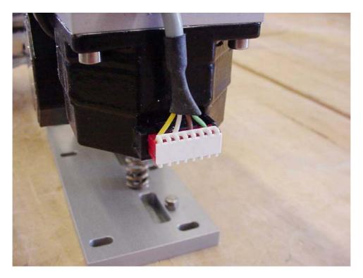
Picture 1: View of connector without any silicone
