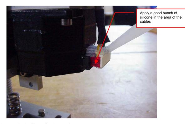
Picture 2: Apply silicone in the are of connectors
