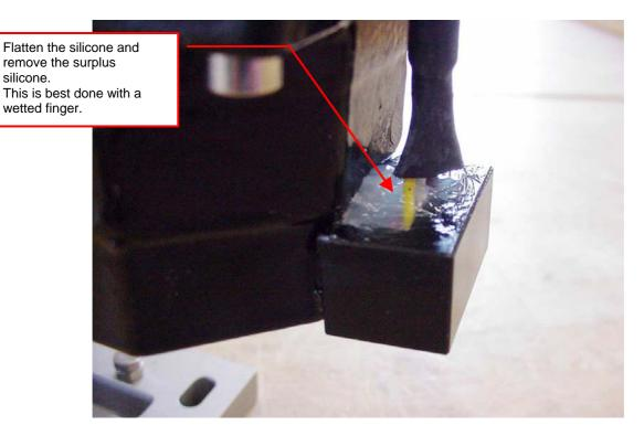
Picture 5: Finished connector sealing
