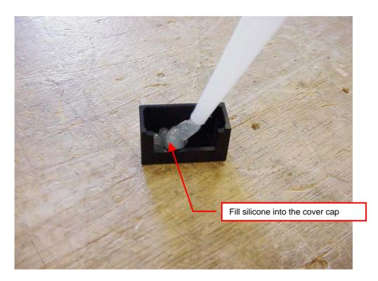
Picture 3: Fill silicone into cover cap
