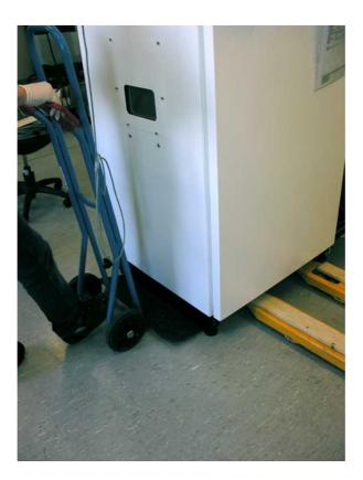
Use sack trolley to lift resp. pull chamber cassis while climate chassis rests on wheel board.
