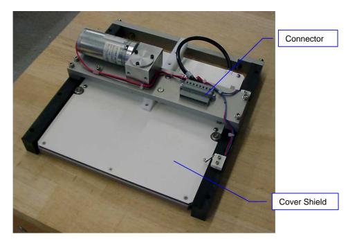
Gate Heater is located under cover shield
