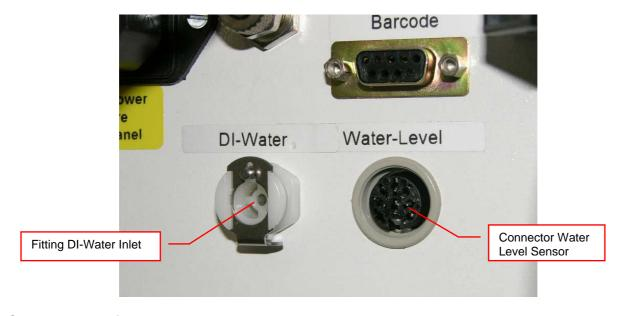
Connect water fitting and water level sensor
