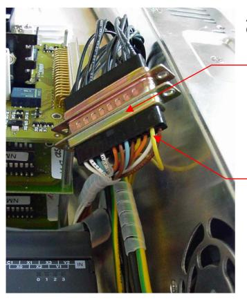
Additional connection from C105.12 to C102.511 when using adaptor:
