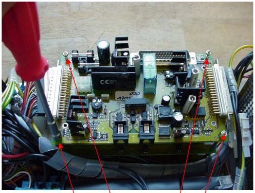
Tighten the 4x M3 Nuts
