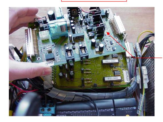
Remove controller board from module
