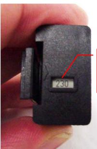
Put the Voltage selector back into the Fuse holder: The supply Voltage should be visible in the little window
