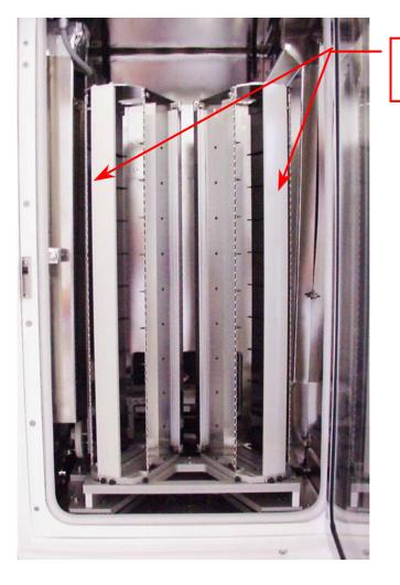
Remove the Stackers from Chamber
