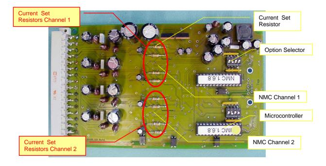
The motor current is set by four resistors per axis. Resistor values must be identical within one axis.
