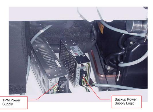
The backup power supply for the logic is connected in parallel to the main power supply. The main power supply feeds into the logic through a diode
