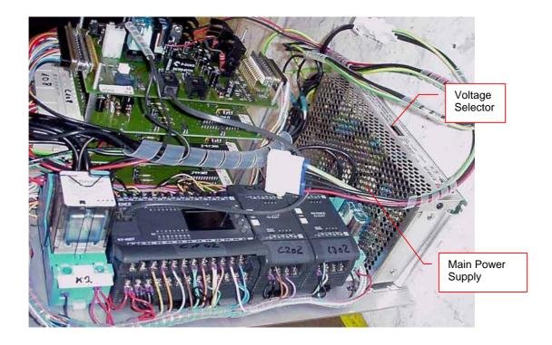
The main power supply is located on the controller module. Early models have a dual voltage power supply with a voltage selector switch. Later models have a wide range power supply with an integrated ventilator.
