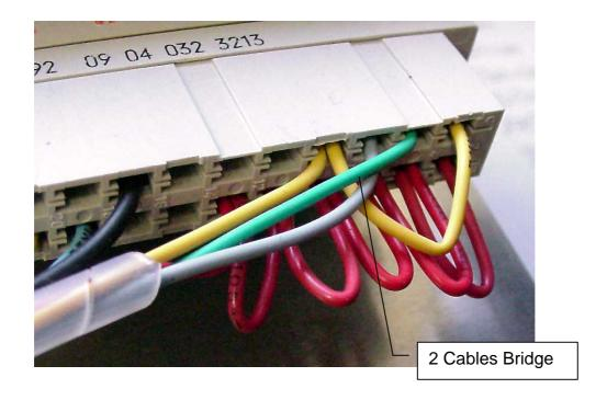
Crimp Contact were taken that are not suitable for two cables.
